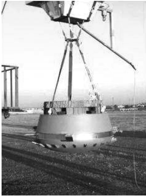
Fig. 1 Integrated mock-up with its different elements (gondola, ring, cone, and upper cover).
